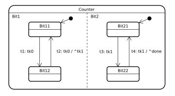
Fig. 2. Model of a two-bit counter
